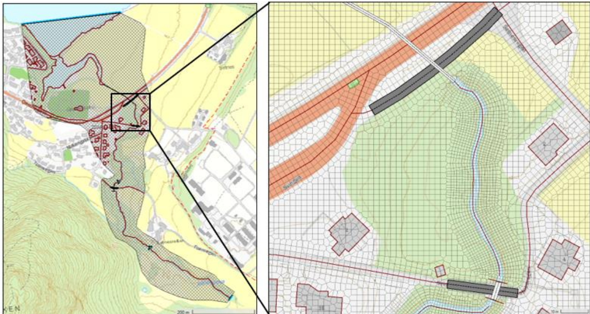
Figur 6-2 Beregningsnett i hydraulisk modell.
